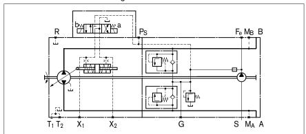
Fig. 14: Hydraulic circuit diagram of A10VG with electric two-point control, with switching solenoid
