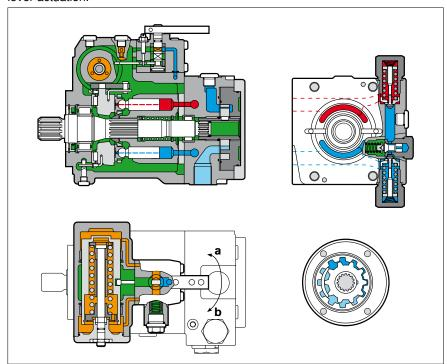
Fig. 7: Cut-away view of A10VG with hydraulic proportional control, mechanical servo
