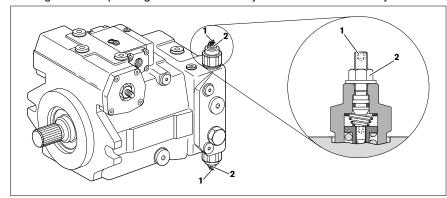
Fig. 15: Activating the bypass function
