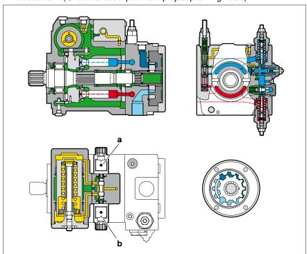
Fig. 10: Cut-away view of A10VG with automatic control, hydraulic, speed related
