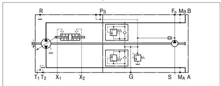
Fig. 9: Hydraulic circuit diagram of A10VG with hydraulic control, direct controlled
