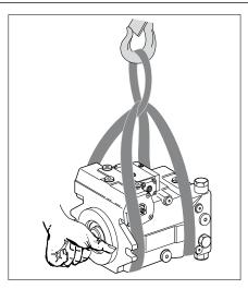
Fig. 18: Transport with lifting strap
