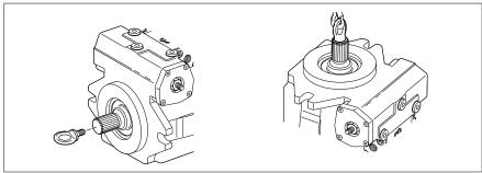
Fig. 17: Fixing the ring screw
