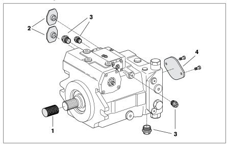
Fig. 1: Axial piston unit
