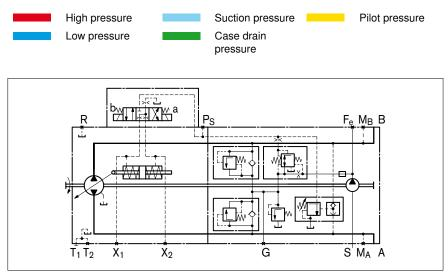
Fig. 11: Hydraulic circuit diagram of A10VG with automatic control, hydraulic, speed related
