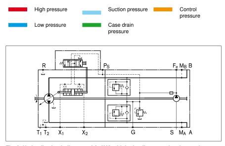
Fig. 8: Hydraulic circuit diagram of A10VG with hydraulic proportional control
