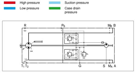
Fig. 4: Hydraulic circuit diagram of A10VG with mechanical trunnion adjustment
