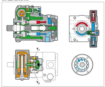
Fig. 5: Cut-away view of A10VG with hydraulic control, pilot-pressure related
