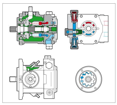
Fig. 3: Cut-away view of A10VG with mechanical trunnion adjustment
