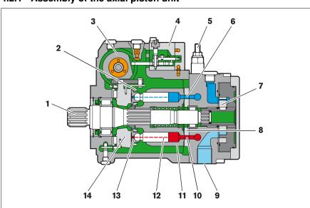
Fig. 2: Assembly of the A10VG series 10
