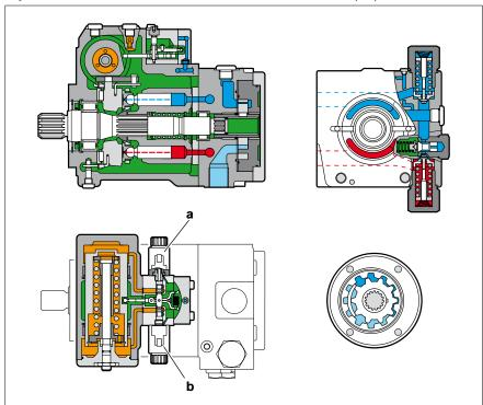
Fig. 12: Cut-away view of A10VG with electric proportional control
